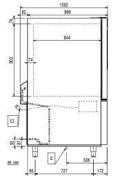
Drain FΙ Electrical inlet (power) Refrigerant Outlet
